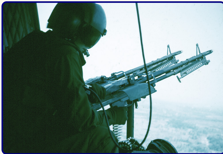
Port twin door-gun airstream deflectors (Image: Roger Buck)
