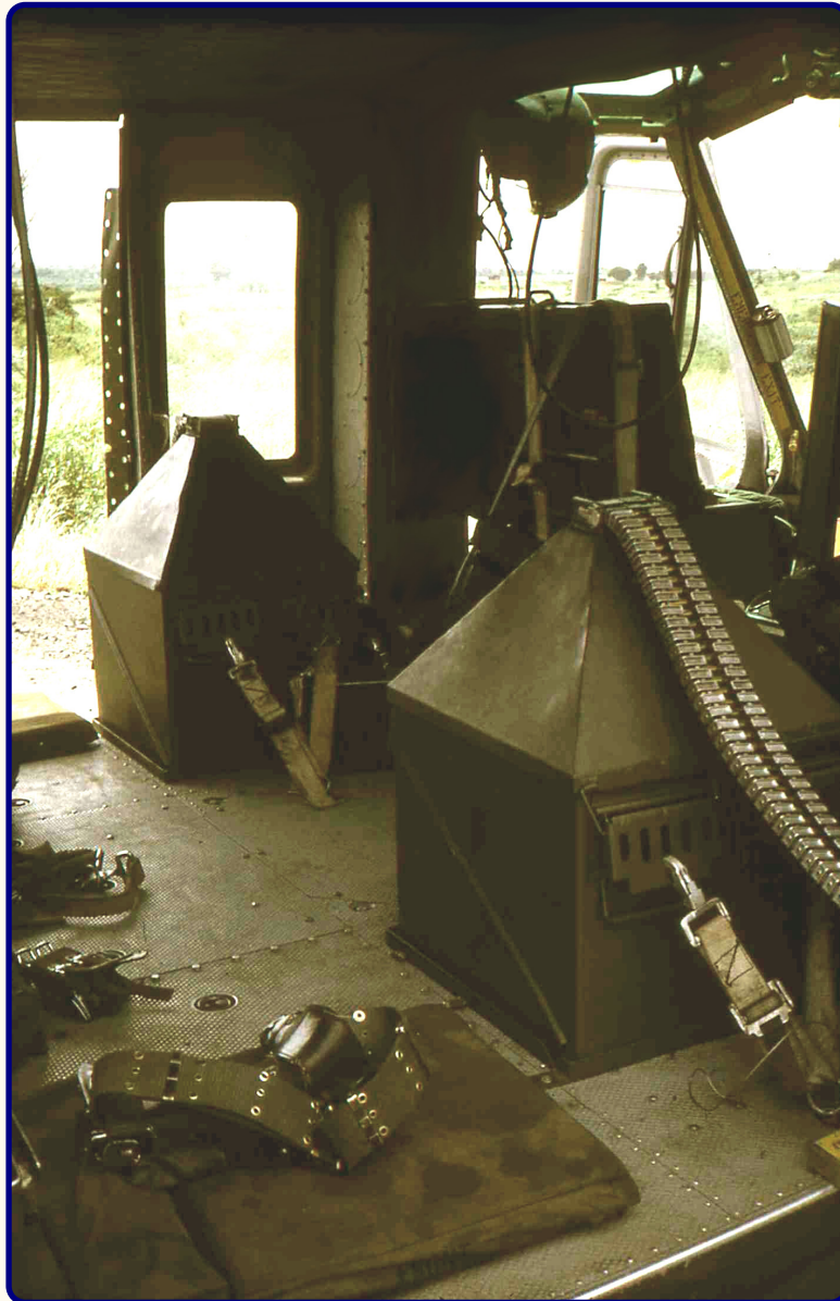
Bushranger hopper-style minigun ammo bins (Image: Norm Goodall)
