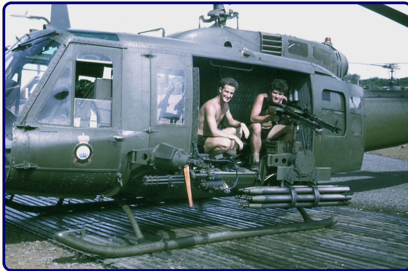
Armed minigun with flagged safety rod (Image: Roger Buck)
