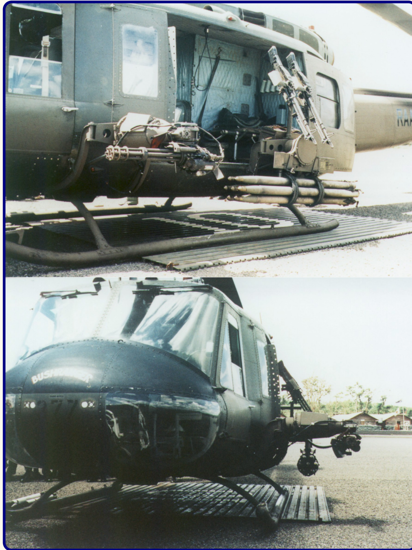
Changed XM21 system configuration showing rocket launch clearance below front pylon (Image: RAAF)
