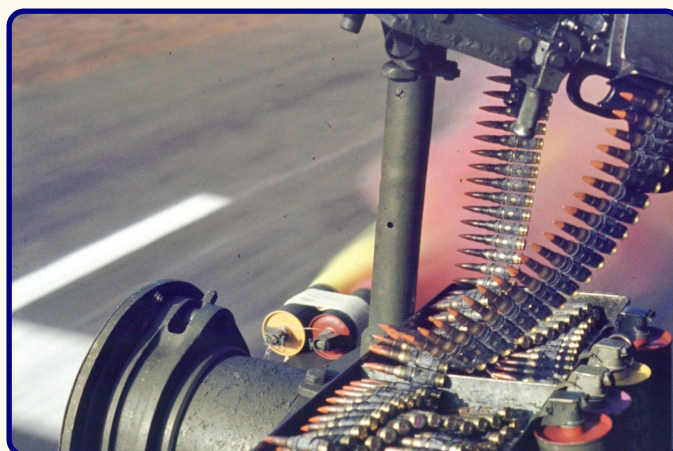
Twin door-gun ammunition bin - capacity 1500 rounds, all tracer (Image: Peter Howe)
