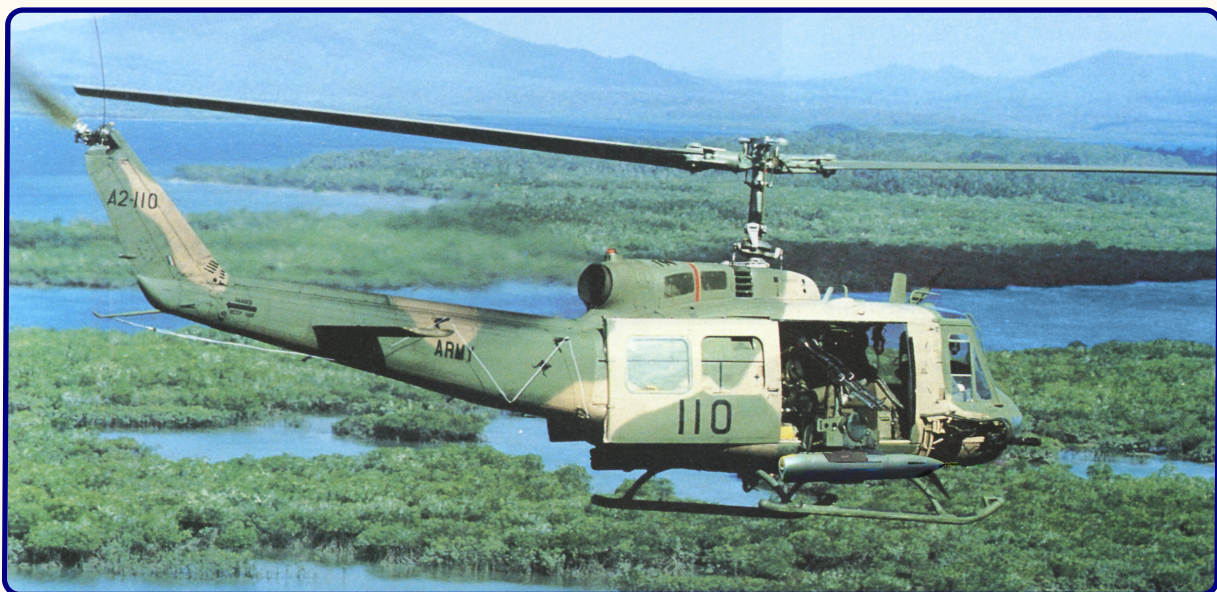
Conceptual ADF Huey II gunship – NC621 20 mm low recoil cannon pods fitted in lieu of 70 mm rocket launchers (Primary image: Australian Army)
