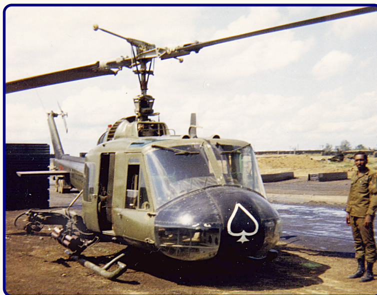
US Army Charlie Model Gunship with XM21 weapon system
