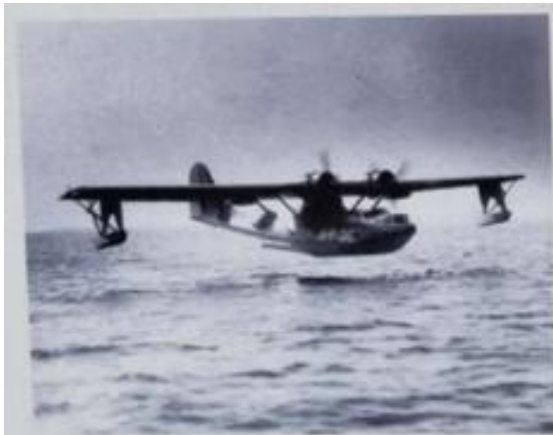
Floats extended for water landing.
