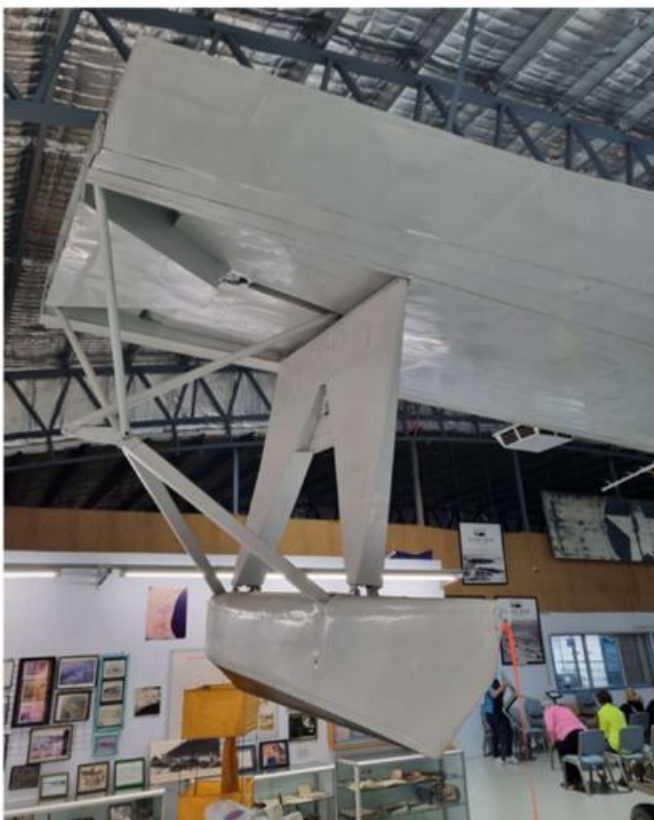
Visible in museum the Catalina wing tip mechanism brings them down to become floats
