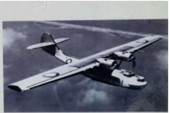
Floats retracted for flight
