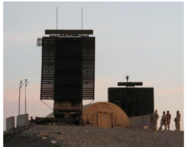
41WG AN/TPS-77 radar at 'Radar Hill', Camp Palomino Kandahar, Afghanistan
