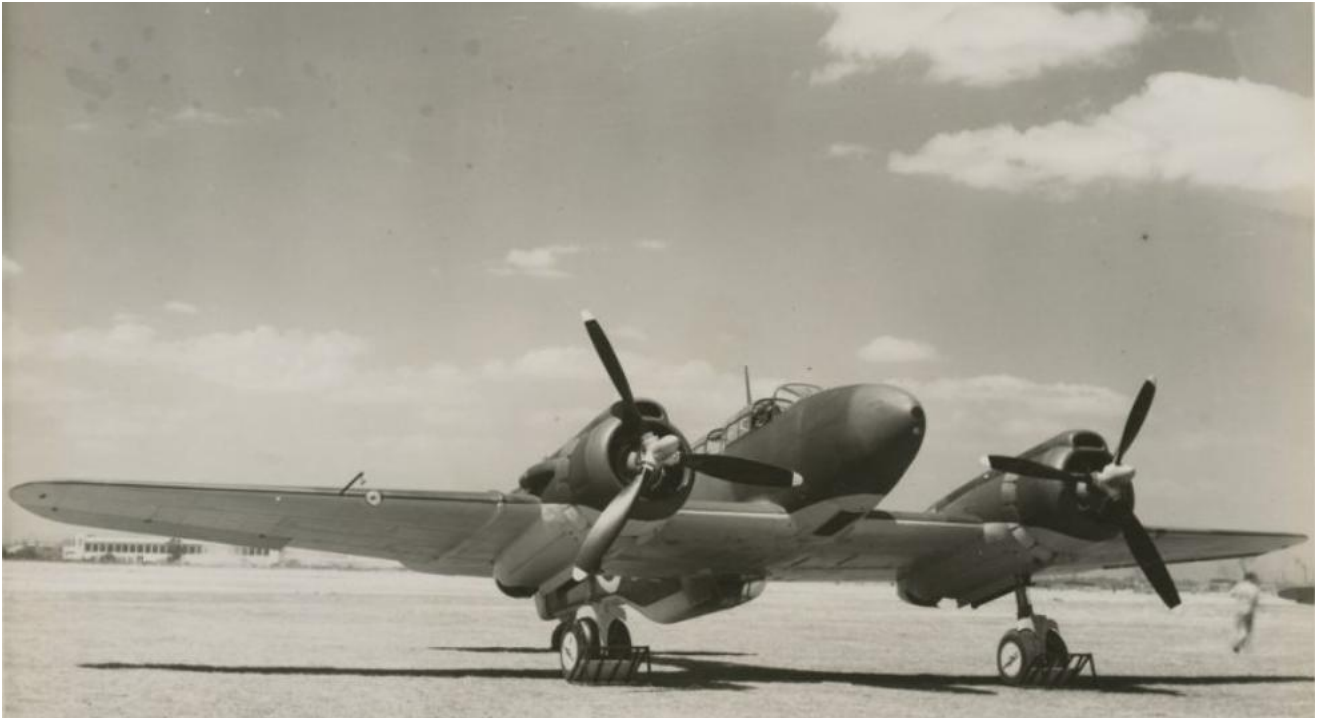
Three-quarter front view of the CA-4 A23-1001 CAC Woomera, prototype of a three-seat strike-reconnaissance and dive-bomber, completed and ready for testing at the CAC factories in Fishermans Bend, Victoria.
