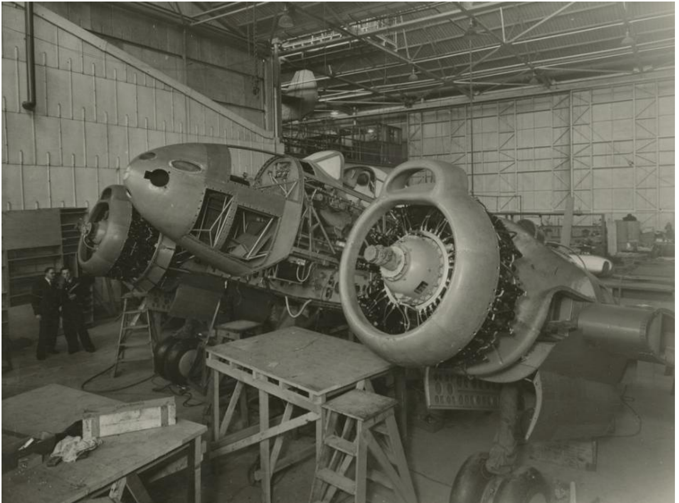
The fuselage and engines of the CA-4 A23-1001 CAC Woomera, a three-seat strike-reconnaissance and dive-bomber, under construction at the CAC factories in Fishermans Bend.
